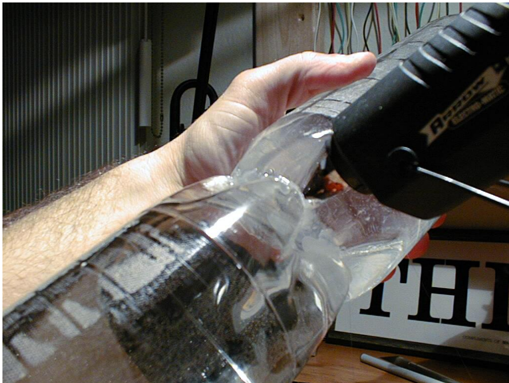
Glue the two bases of the pop bottle together. Many different types of adhesives have been used in the past with great levels of success. A flexible hot glue is preferred by the Professor because it hardens quickly which allows rapid construction.
